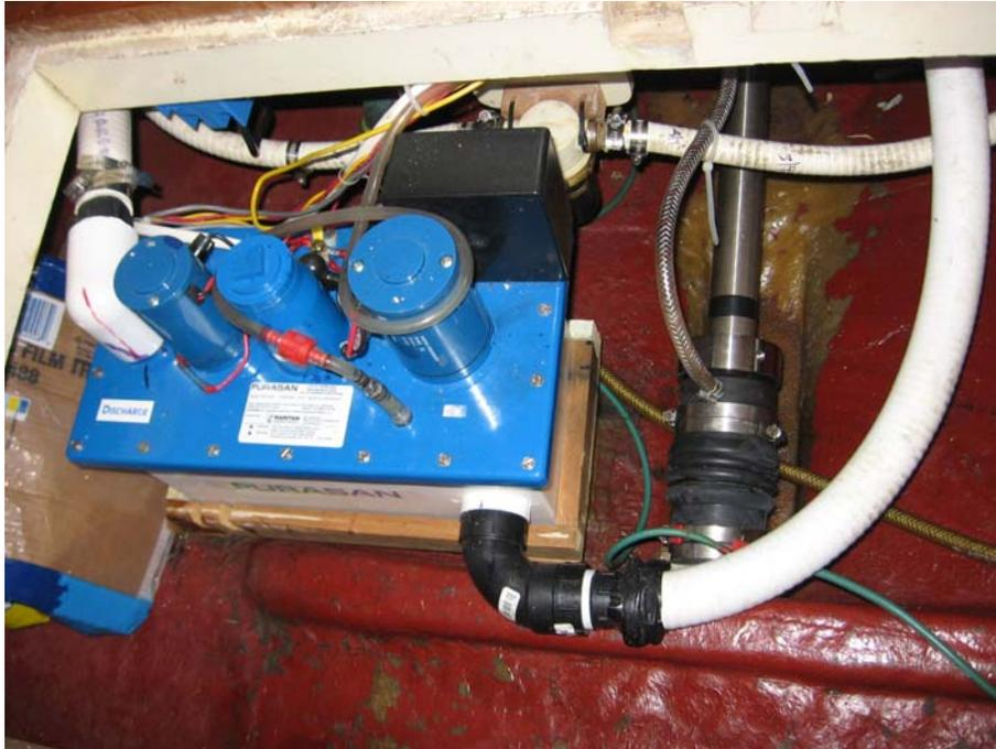
Picture #1 Purasan Treatment Tank installation on SAY GOODBYE
