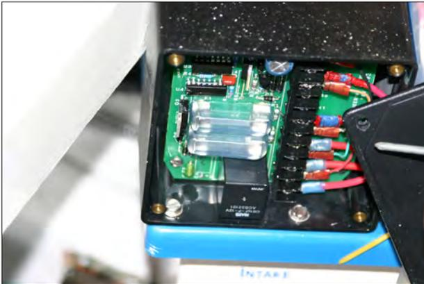
Now remove the two 5/16" head screws in the bottom of the black box that hold down the treatment tank lid. Loosen and remove the locknuts underneath the screws with a 3/8" wrench.
