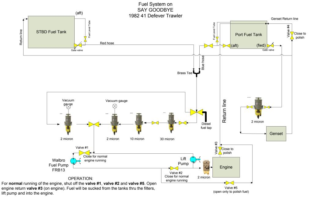
To prime the system or use the Walbro as a lift pump...open the valve #1 before the Walbro and valve #2. Close valve #5. The Walbro will feed the engine.
